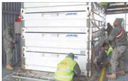
Soldiers from the 39th Transportation Battalion's Movement Control Team secure a stack of four portable housing units to a T3 pallet train of three 463L Air Force pallets. The entire mission, which required a total of 18 C-5 Galaxy aircraft flights, was completed Feb. 18.
