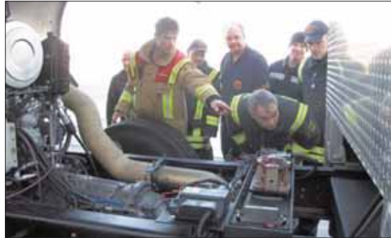
USAG Heidelberg firefighter Thorsten Stuerz (right) gets a close look as Stefan Groetschel, chief of the IMCOM-Europe and USAREUR Firefighting Training Center at USAG Ansbach Fire Department (left), explains preventive maintenance checks and inspection procedures on the transmission of the new newly refurbished fire truck to USAG Heidelberg firefighters during initial training session.
