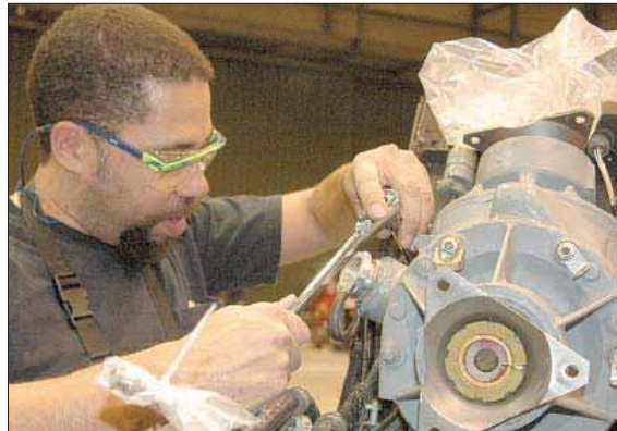
(Above) Dyncorp International employee Richard Clark tightens a bolt on a UH-60 Black Hawk tail rotor intermediate gear box. (Left) A Dyncorp International employee pours an adhesive to repair a pilot's floor panel in a UH-60 Black Hawk.
