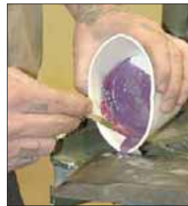
(Above) Dyncorp International employee Richard Clark tightens a bolt on a UH-60 Black Hawk tail rotor intermediate gear box. (Left) A Dyncorp International employee pours an adhesive to repair a pilot's floor panel in a UH-60 Black Hawk.
