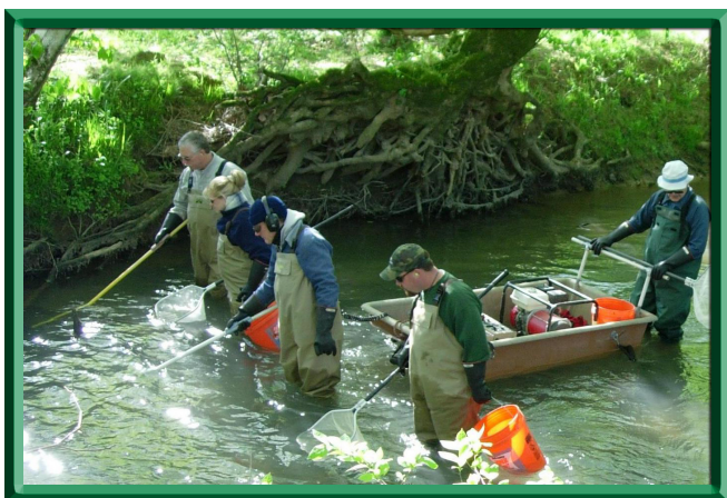
Electrofishing equipment is used to collect fish for community assessments, bioindicator studies, and contaminant analyses.
