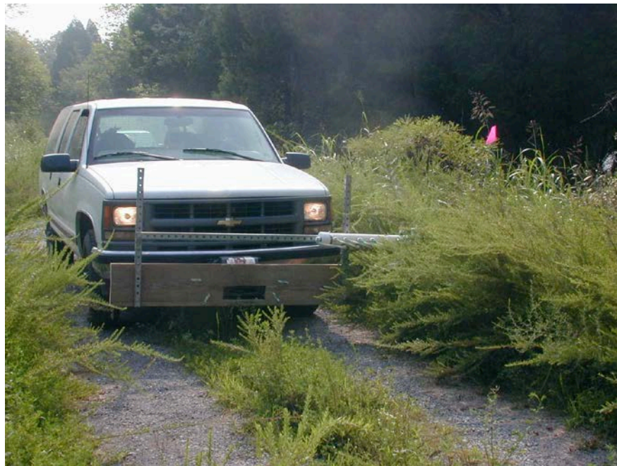
Fig. 5. Truck-mounted wick-type herbicide application device being used to apply glyphosate-based herbicide to lespedeza and Johnsongrass at the Raccoon Creek Barrens.
