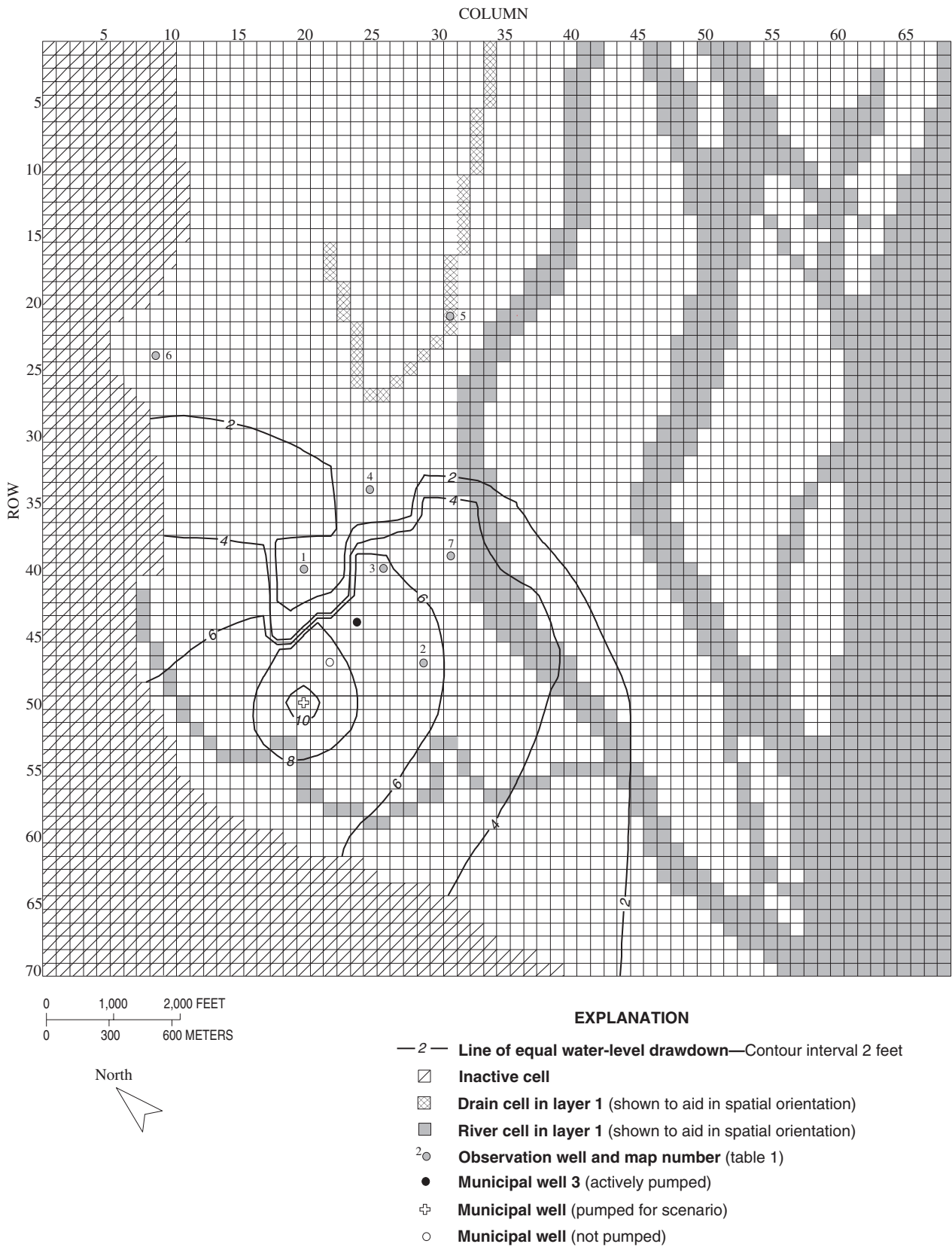
Figure 11. Simulated drawdown in layer 2 of the flow model from hypothetical pumping of a second existing City of Burlington municipal well.
