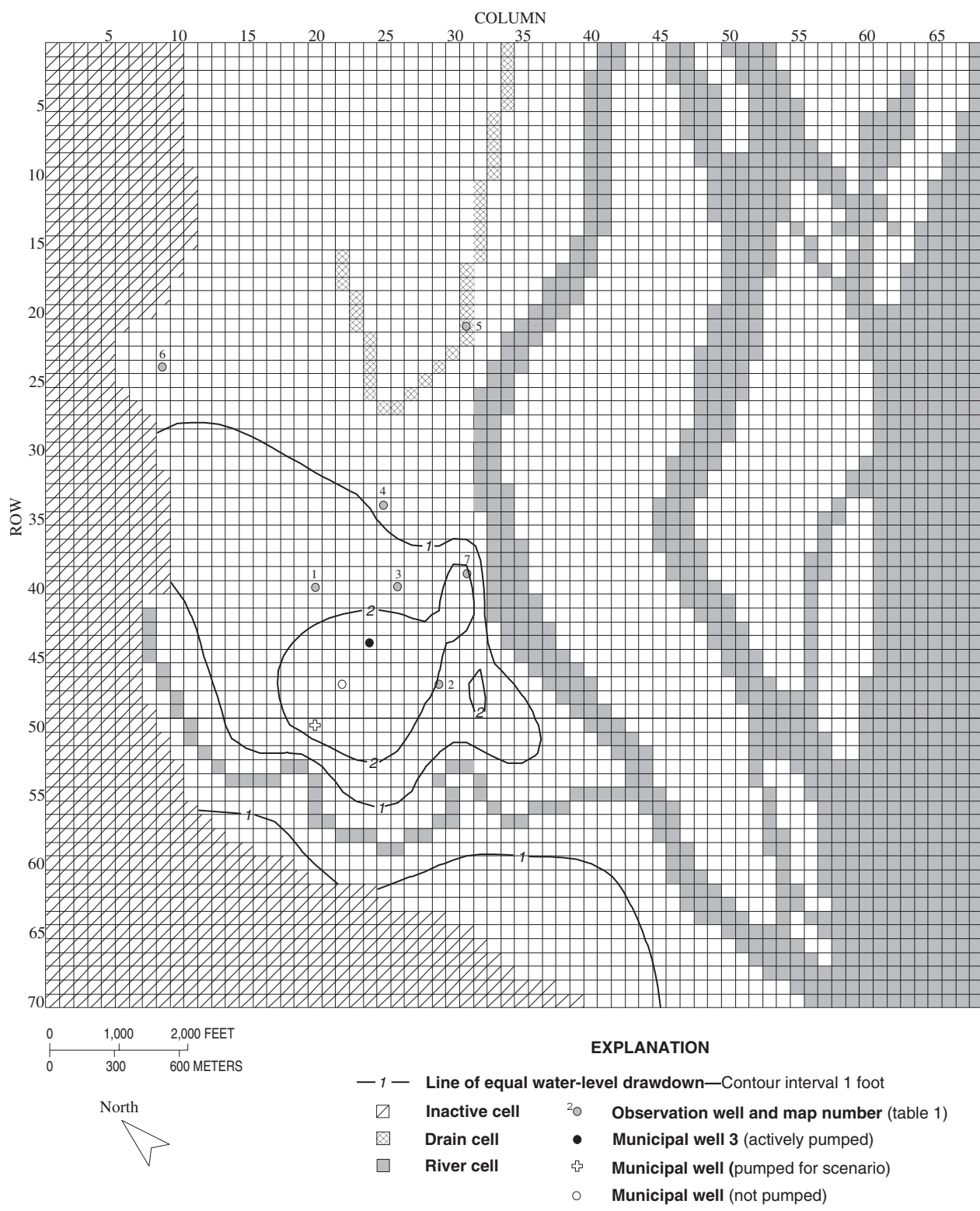
Figure 10. Simulated drawdown in layer 1 of the flow model from hypothetical pumping of a second existing City of Burlington municipal well.
