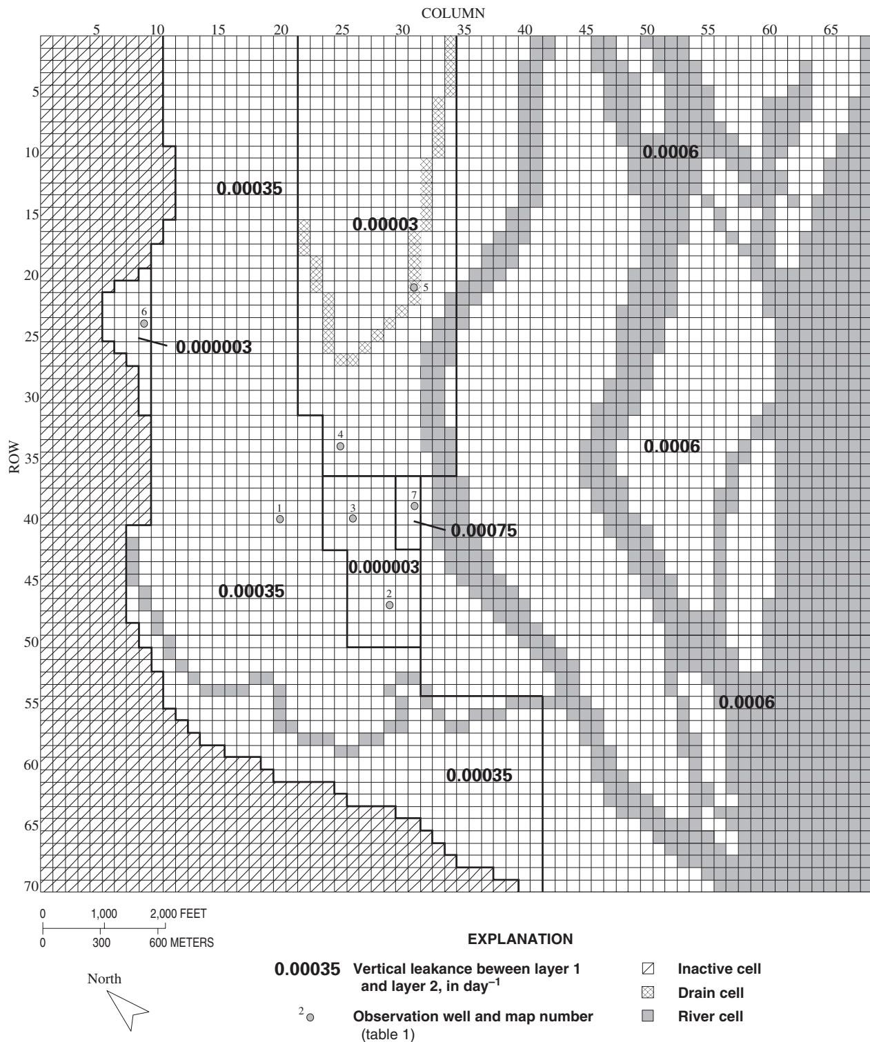
Figure 7. Vertical leakage assigned to cells between layer 1 and layer 2 of the flow model for the Mississippi River alluvium near Burlington, Iowa, 1999.
