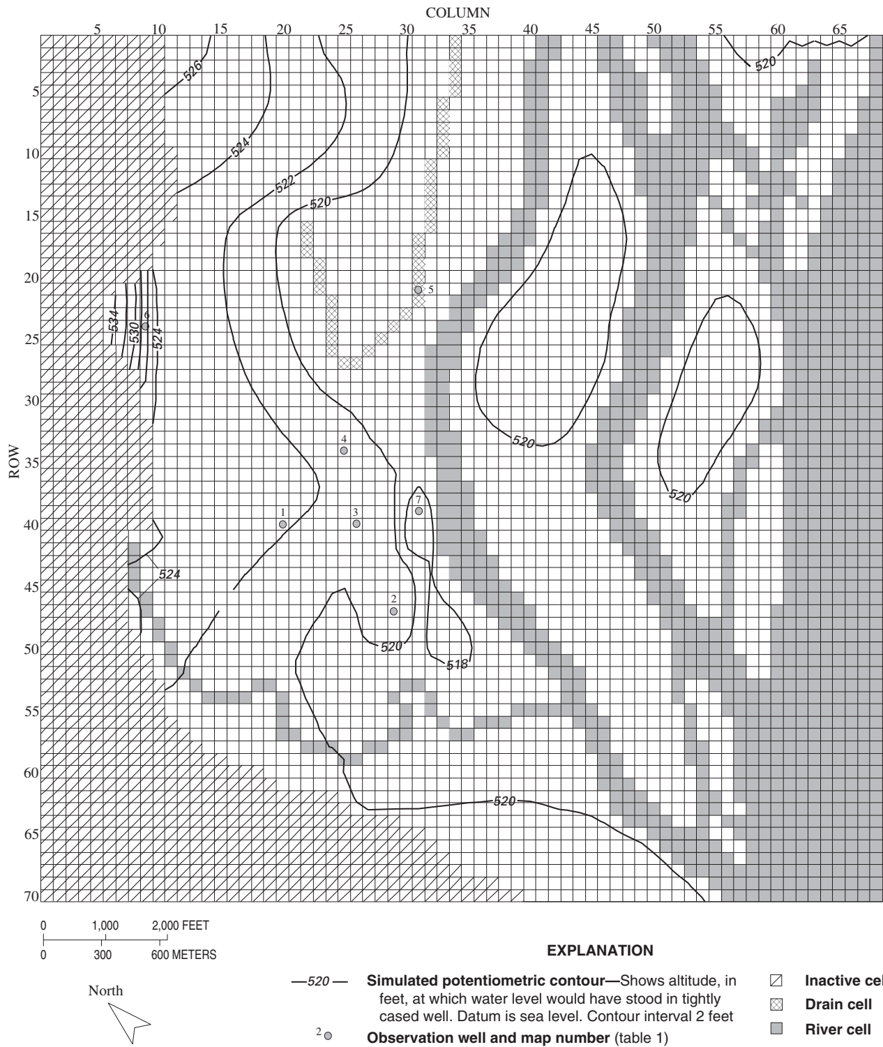
Figure 8. Simulated potentiometric surface in layer 1 of the flow model for the Mississippi River alluvium near Burlington, Iowa, October 1999.
