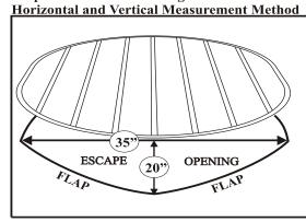
If measured by the current method the proposed escape opening would be at least 35 inches (89 cm) in horizontal taut length and simultaneously, 20 inches (51 cm) in vertical height at the exit opening cut.
