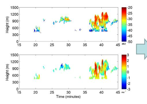
Sample 30-min period showing the reflectivity (top) and mean Doppler velocity as observed by AMF cloud radar
