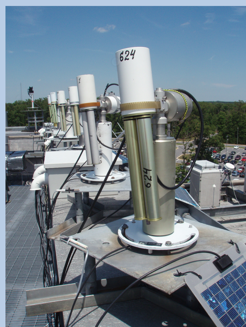
Richard Wagener(2010): AERONET outdoor calibration facility at NASA Goddard Space Flight Center during a visit on 2010-07-26. A few of the dozens of CSPHOTs that can be intercalibrated simultaneously.
