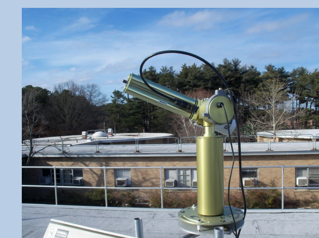
Laurie Gregory (2011): CSPHOT on top of Bldg. 490 at BNL doing a direct Sun observation.
