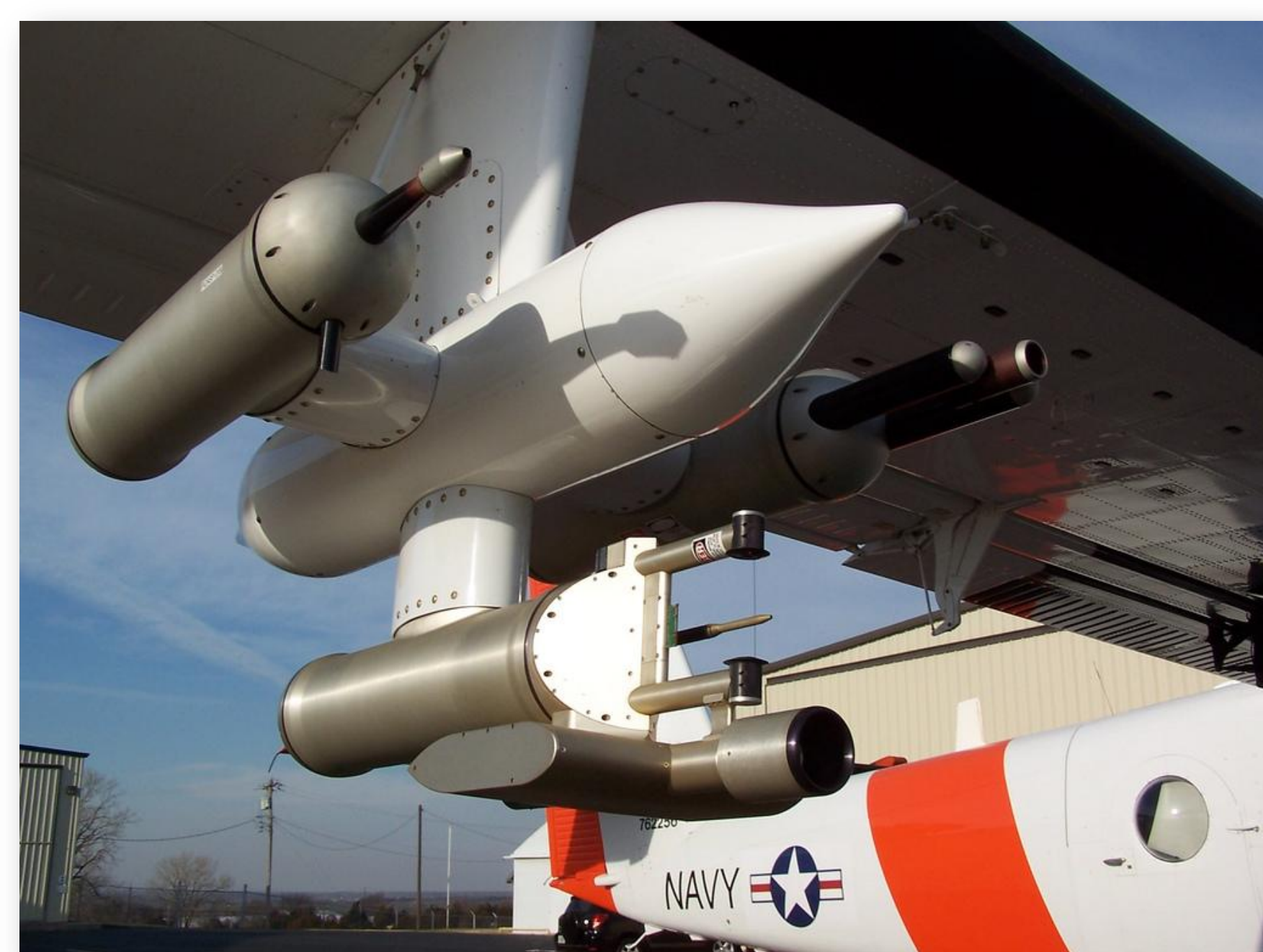
Figure 1. Measurement probes mounted under the wing of the CIRPAS Twin Otter aircraft. (Photo from ARM)
