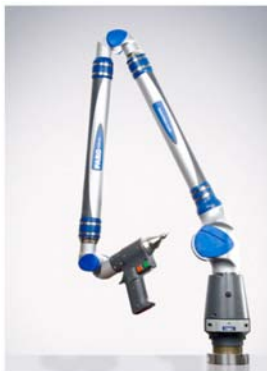
Faro arm used to measure edge position
