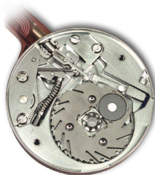
A mechanical safe arming detonator (MSAD) prevents accidental or unintended detonation of a nuclear warhead. Stockpile stewards at Livermore are working on an advanced MSAD for the W78.
