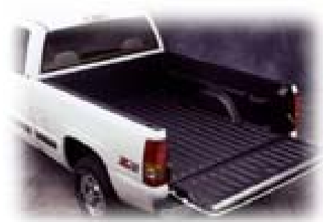
Figure 4. The Chevrolet Silverado pickup truck box and tailgate, manufactured from SRIM composite, were released to the public as an option in 2001.
