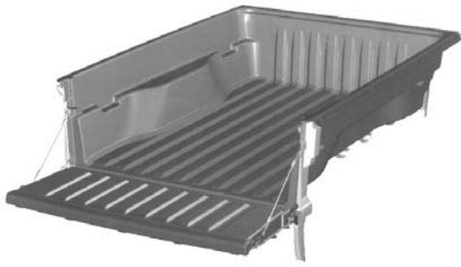
Figure 1. Computer-aided design of the truck box and tailgate. Ribs add strength and stiffness.
