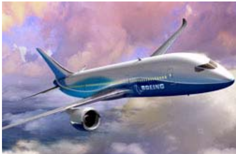
Figure 5. Boeing’s 787 “Dreamliner” uses SRIM composites for structural parts, increasing fuel efficiency by 3 percent. Overall fuel savings is 20 percent compared with the 747. Its first commercial flight is anticipated in 2008.
