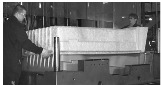
Figure 2. Loading a glass fiber preform onto the molding tool in preparation for polyurethane injection. For high-volume production the loading could be automated.
