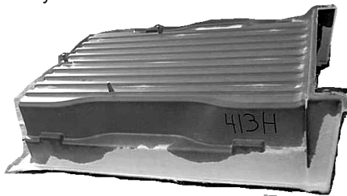
Figure 3. Example of an incompletely filled box molding, which was a result of too little pressure.
