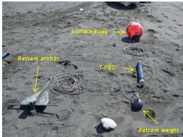
Figure 2a: Standard mooring line with surface buoy. Figure 2b: Mooring without surface buoy.
