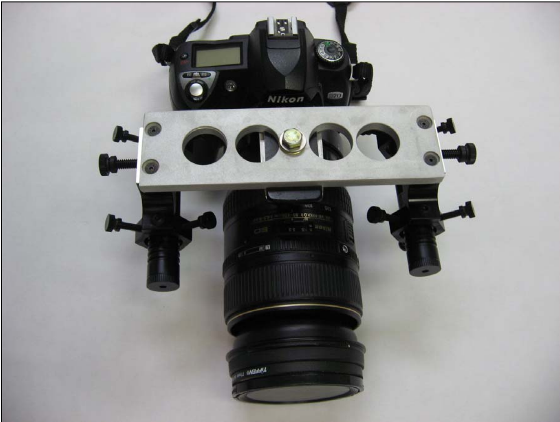
Figure 5. Two laser-pointers were mounted horizontally in parallel by an aluminum bracket attached to the tripod-mount of a Nikon 80-400 mm zoom lens.
