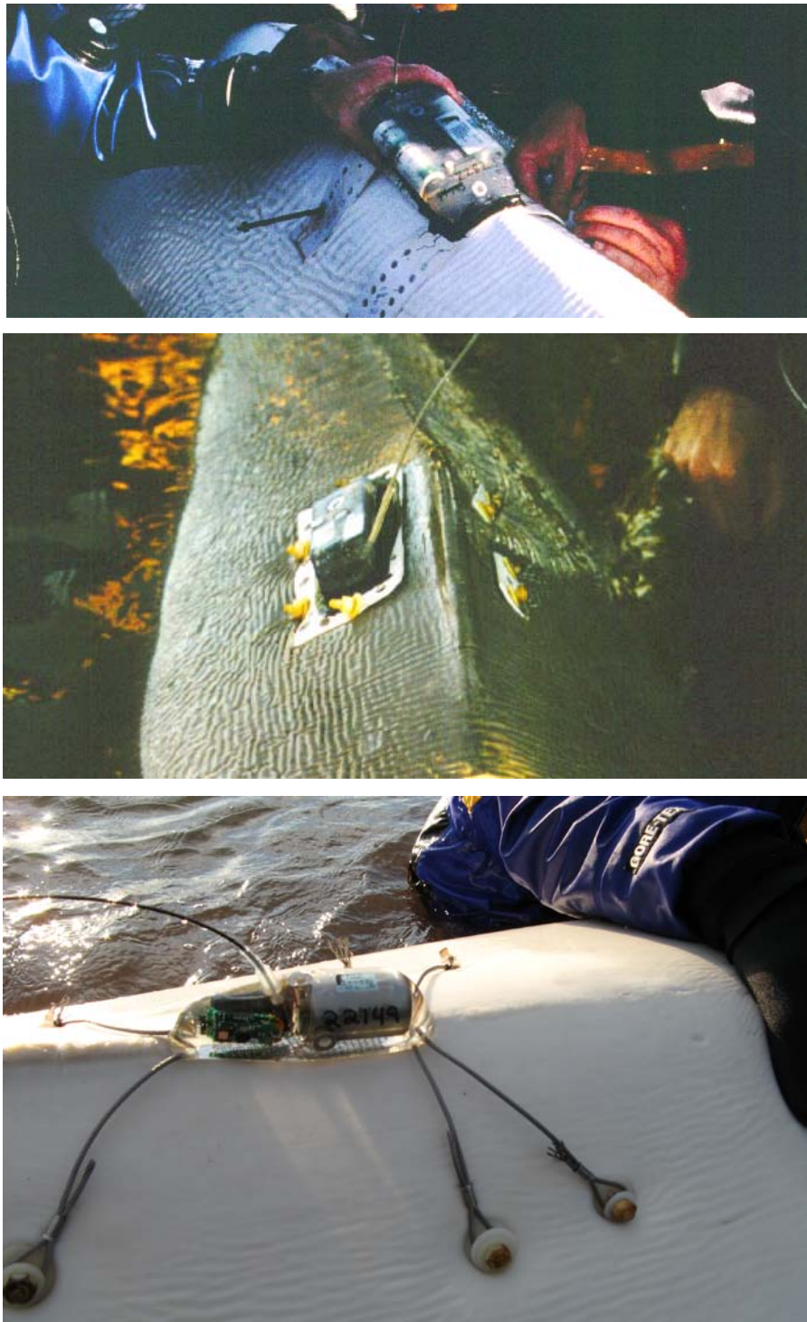
Figure 4-1. Configurations of satellite data recorders deployed on beluga whales in the eastern Chukchi Sea in 1998, 1999, 2001, 2002, and 2007. Upper panel: saddle tag. Middle panel: side mount. Lower panel: spider tag.
