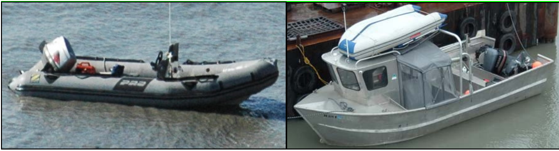
Figure 6. The two vessels used to survey beluga whales in Upper Cook Inlet, Alaska. The R/V Leucas, left, is a Zodiac ProMan 9, 16 ft (4.9 m) rigid-hull inflatable that was used in 2006 and 2007, and the R/V Nerka, right, is a 26 ft (8 m) aluminum craft was used in 2006 only. Both vessels were equipped with 4-stroke Yamaha motors (50 hp and 250 hp, respectively) during the summer of 2006.
