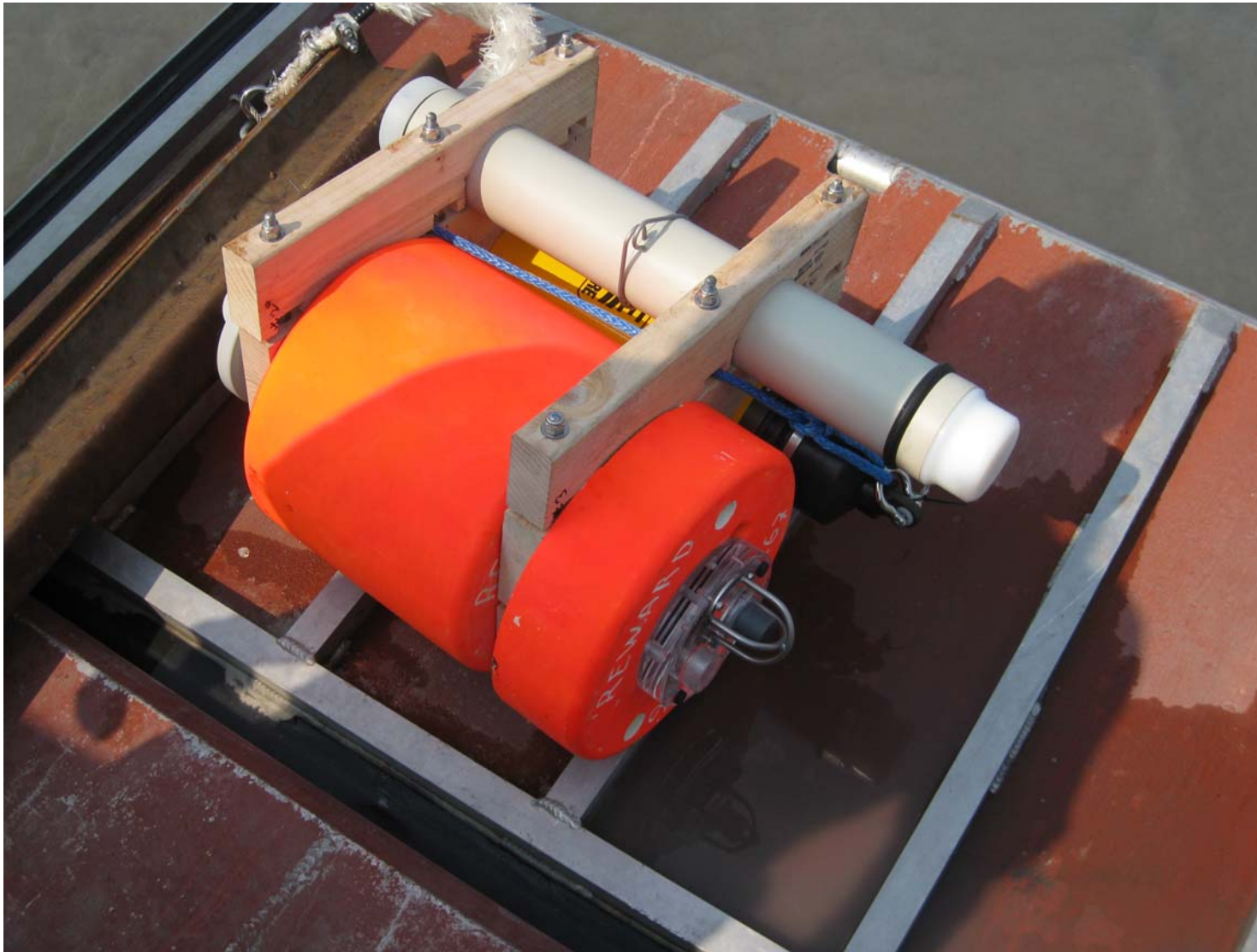
Figure 3. The acoustic mooring design used at the Eagle River location, with the C-POD (grey tube), EAR (inside the orange syntactic foam collar), and acoustic release (under the C-POD) held close together by a wooden frame. The white mooring line (top, left of center) attaches the acoustic equipment to the railroad track used as an anchor.
