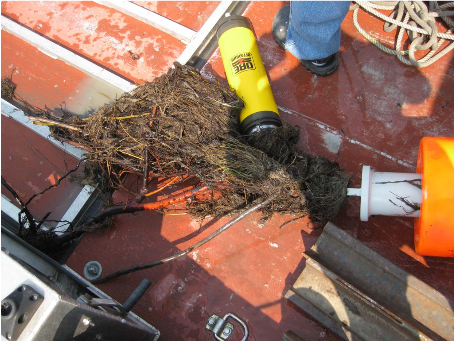
Figure 2. Vegetative debris on the mooring line between the acoustic release (yellow) and EAR (grey) on the Eagle River – South mooring.
