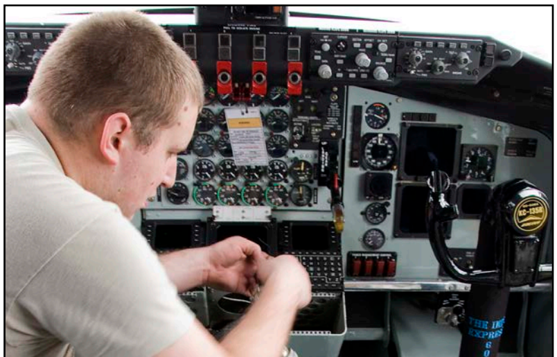
RIGHT: Staff Sgt Gregory Lee and Senior Airman Matthew Steele, both 434th Aircraft Maintenance Squadron electrical and environmental systems technicians, use a tablet device while tracking down a wire causing intermittent failure issues with a KC-135's the fuel dump actuator.
