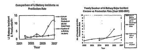
As illustrated by the graph on the left, the number of documented lithium battery incidents significantly increased in between 2005-2007. The incident rate was compared to the production rate of lithium cells during the same time period. Though the number of incidents increased faster than the production rate, the small number of incidents made it difficult to draw any conclusion about a causal relationship between production rates and incident trends. —
