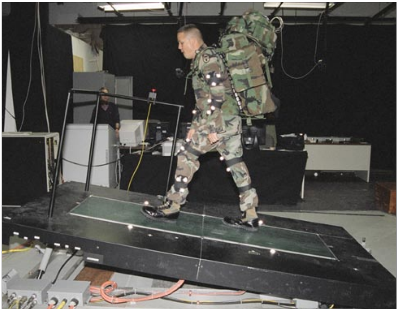
Spc. Hipolito Ramos walks on the Force Sensing Treadmill in the biomechanics lab. Hydraulic lifts adjust the platform up to a 25 percent uphill or downhill grade without stopping the belt or test subject.
