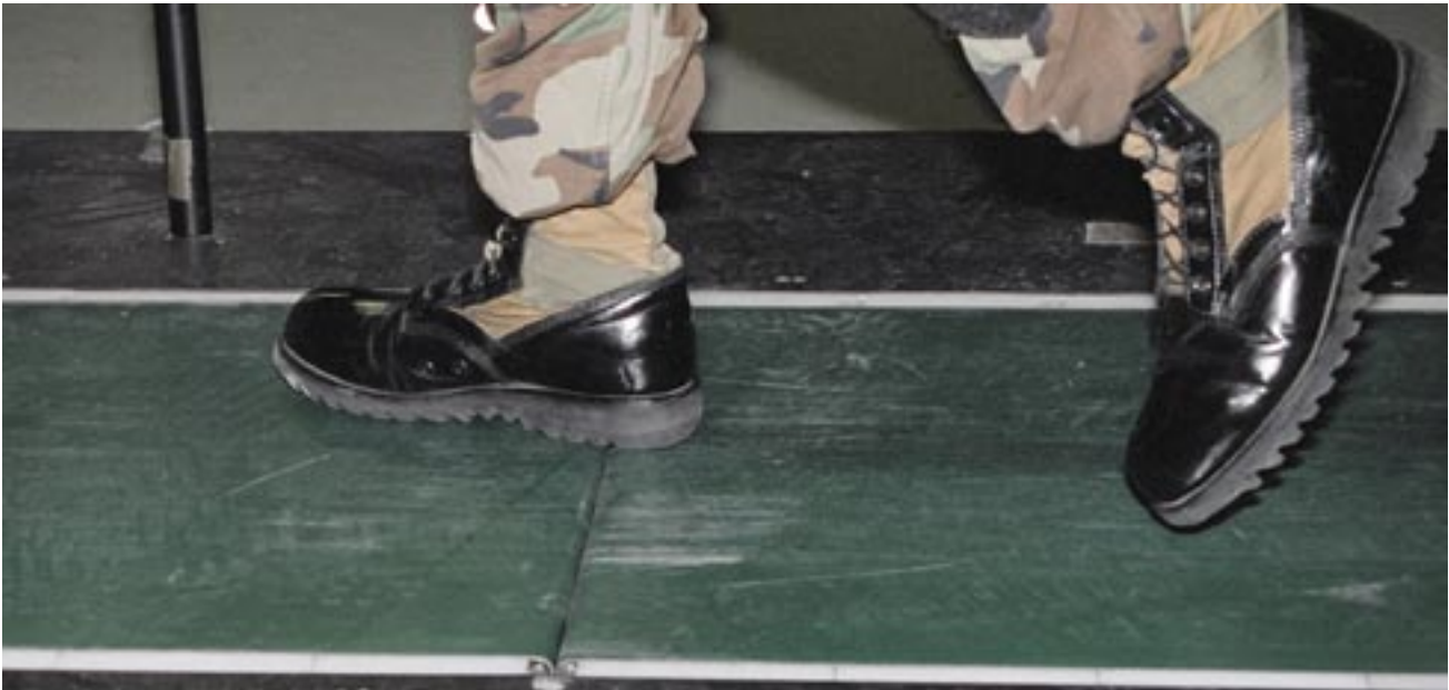
Dual belts on the Force Sensing Treadmill gather 3-D force data separately for each foot.
