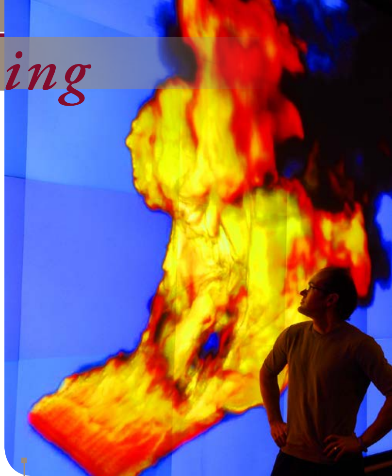
Stefan Domino studies a rendering of a simulated jet fuel fire in a crosswind displayed at Sandia's Joint Computational Engineering Lab. The 400-million-variable simulation helped engineers prepare an experiment at Sandia's Thermal Test Complex.
