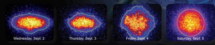
First results from NIF experiments in September 2009 successfully demonstrated the use of wavelength tuning to adjust the shape of the target capsule implosion from asymmetric to spherical, a key requirement for achieving ignition.
