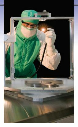
Together with two industry partners, LLNL developed a novel continuous melt process for manufacturing the more-than 3,000 meter-sized slabs of ultrahighquality neodymiumdoped phosphate laser glass needed for NIF.
