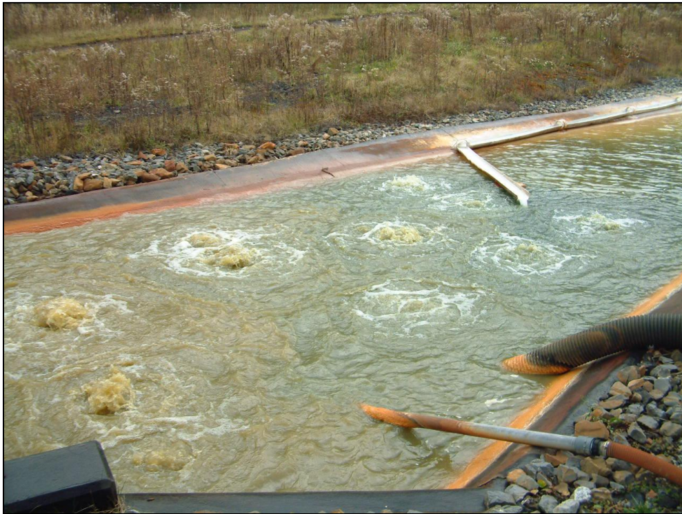
Figure 22. Aeration of the mine water after lime addition. The greenish color is caused by ferrous iron.
