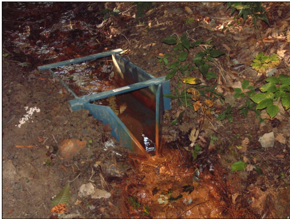
Figure 28. H-type flume below the Shawmut Mine portal.
