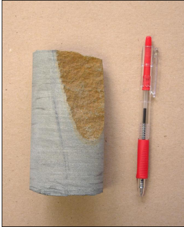
Figure 20. Interburden core sample exhibiting high-angle subsidence-induced fracture in a siltstone unit with iron staining due to ground water contact.
