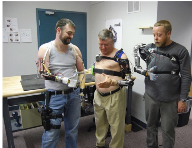
Users wear and control, without surgery, an advanced prosthetic arm developed under the Defense Advanced Research Projects Agency's Revolutionizing Prosthetics program. (Courtesy photo)
