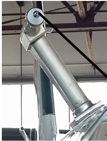
CVI inlet (aerosol from evaporated cloud particles when in clouds)
