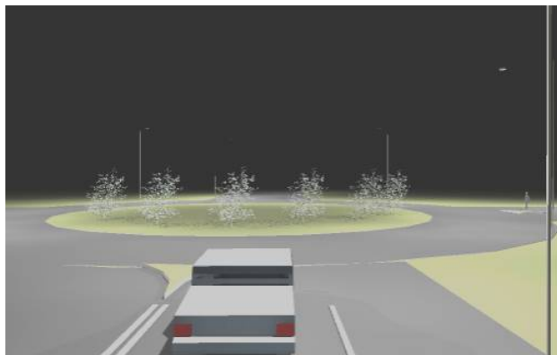
Figure 12. Rendered image of the roundabout with conventional pole-mounted illumination, and with vegetation present. A passenger vehicle is shown in the foreground
