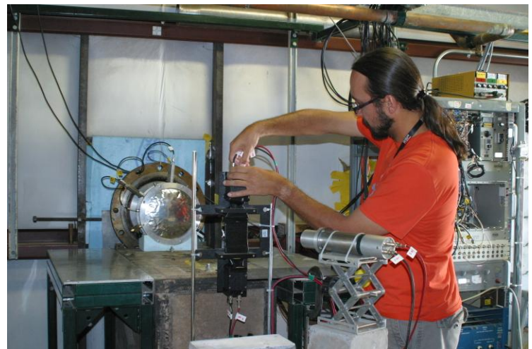
Adjusting active sample for n-p capture experiment on 15R flight path
