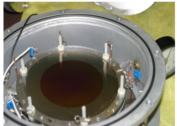
Picture of a fission chamber with the front window removed. A U-235 foil is seen in the center.
