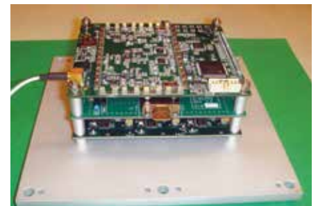
The electronics assembly of a Cornell designed and built scientific–grade GPS receiver that measures TEC (Total Electron Content). The MICA payload provided the first space flight opportunity for this new science instrument.
