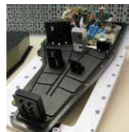
Figure 3 –The Dual Grating Spectrometer flown on flight 36.263
