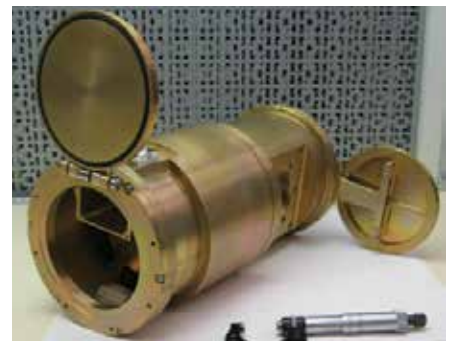
Figure 2 –The Optics Free Spectrometer flown on flight 36.263
