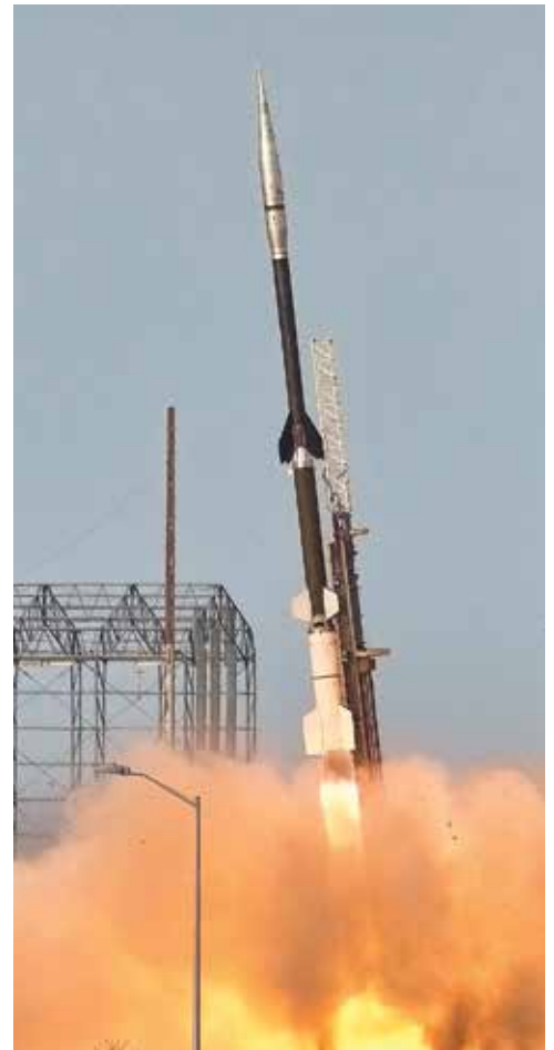
IRVE–3 launches from Wallops Island onboard a three stage Black Brant XI sounding rocket.
