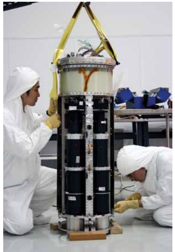
Fig. 2 b. Preparing the instrument for flight. The optics and detectors are cooled by liquid nitrogen to -196\text{ C} ( 77\text{ K} , -321\text{ F} ) during the flight to eliminate infrared emission from the instrument and to achieve the best detector sensitivity.
