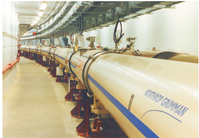
Relativistic Heavy Ion Collider (RHIC) at Brookhaven National Laboratory. The machine itself is enclosed in a tunnel, 12 feet under the ground. Inside two tubes, ion bunches race around RHIC's 2.4-mile ring in opposite directions.
