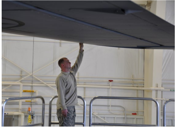
Master Sgt. Jason Lawson, 507th Air Refueling Wing maintenance squadron checks the distance between the new KC-135 maintenance platforms and the wing of a KC-135. The new platforms are expected to increase safety during Isochronal Inspections. (Photo by Senior Airman Mark Hybers)
