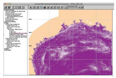
GNOME can use models on a variety of grids, including rectangular, curvilinear, and triangular grids. Here, current data for the Gulf of Mexico from Naval Research Laboratory's NCOM (Navy Coastal Ocean Model) has been loaded into GNOME. Global NCOM (based on the Princeton Ocean Model) is a 1/8-degree resolution operational nowcast-forecast system on a curvilinear grid.
