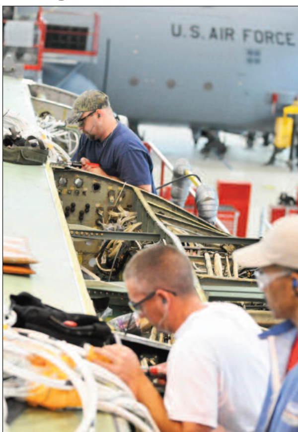
Top to bottom, Jonathan Hampton, Mike Pickens and Sam Wiggins, 402nd Aircraft Maintenance Group, work to attach the main vertical beam onto a new C-130 center wing box. The C-130 Programmed Depot Maintenance Team at Warner Robins Air Logistics Complex became part of the AFSC in July.
