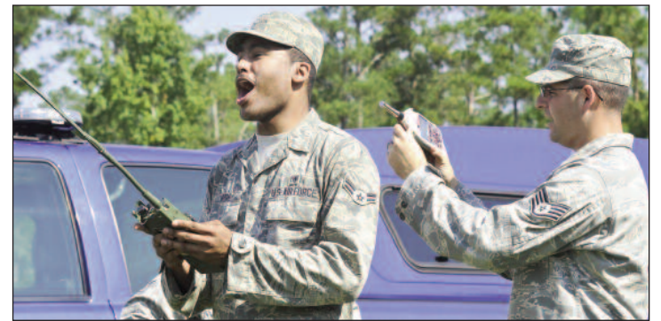
U.S. Air Force photos by MASTER SGT. ROGER PARSONS Airman 1st Class Bruce Moore, 78th Medical Group bioenvironmental engineer, gives a 'fire in the hole' warning prior to setting off an explosion, while Staff Sgt. Barham Bratton, 78th MDG bioenvironmental engineer, takes a noise dosimeter reading.
