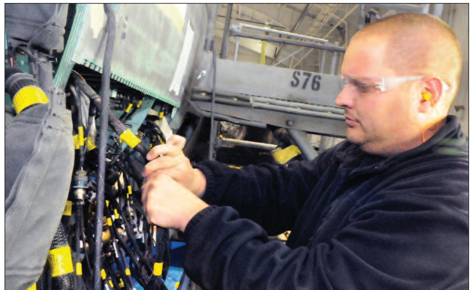
U.S. Air Force photo by SUE SAPP Lee Garvin, 561st Aircraft Maintenance Squadron, works on the rewire of an F-15.
