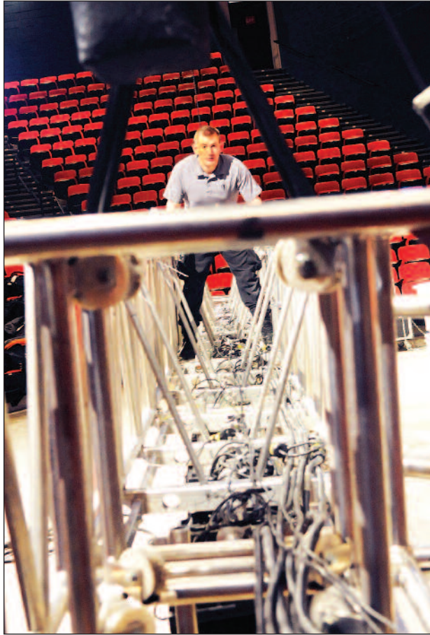
Above, Airman 1st Class Kegan Davis, Tops in Blue lighting director, sets up the front lighting truss.
