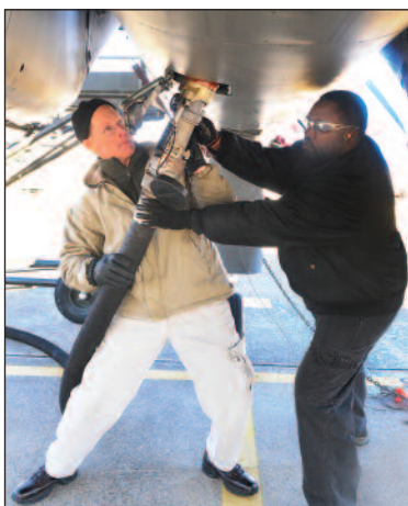
U.S. Air Force photo by SUE SAPP David Witte and Dexter Jefferson, aircraft mechanics, connect a refuel cart to purge an F-15.
