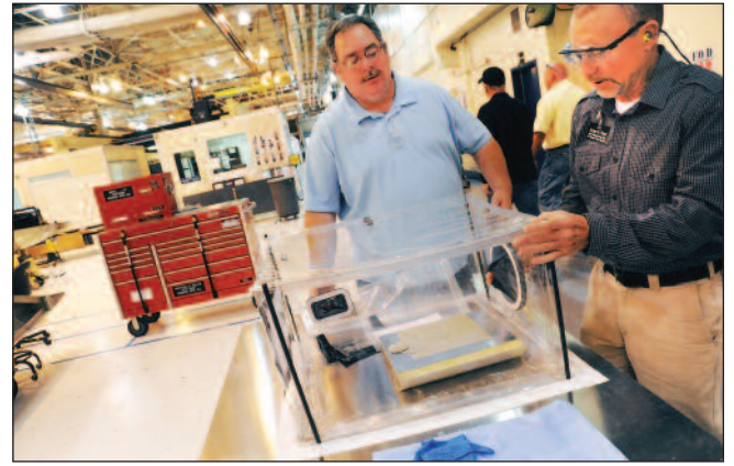
George Pierce, right, 574th Composite Repair Flight director, and Ray Fisher, sheet metal worker; discuss advantages of containment bags which help reduce dust migration.
