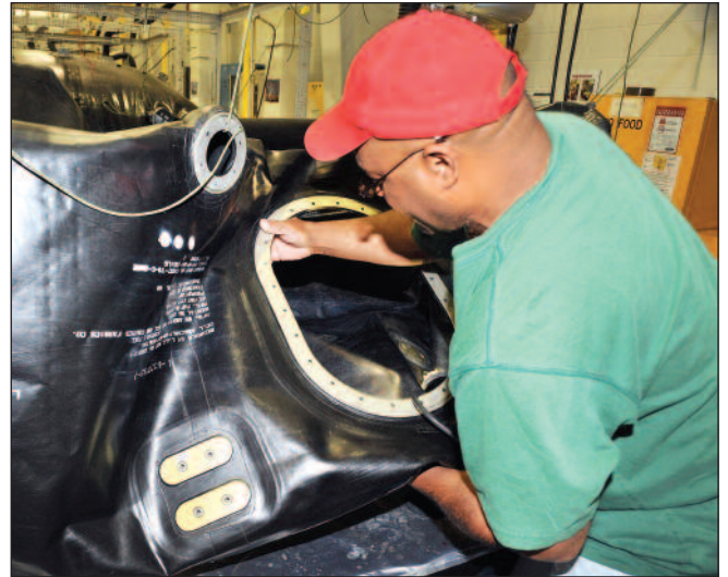
Lyndon Baines Johnson, 402nd Commodities Maintenance Group Fuel Cell Repair Shop mechanic, inspects a fuel cell bladder. Johnson came up with a new process of repairing and replacing the bladders which helped solve an OSHA citation.
