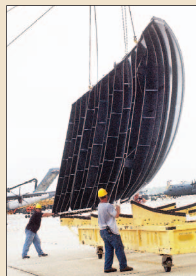
U.S. Air Force photo by SUE SAPP C-5 maintainers guide a C-5 aft cargo door from a crate onto a cradle July 27.
