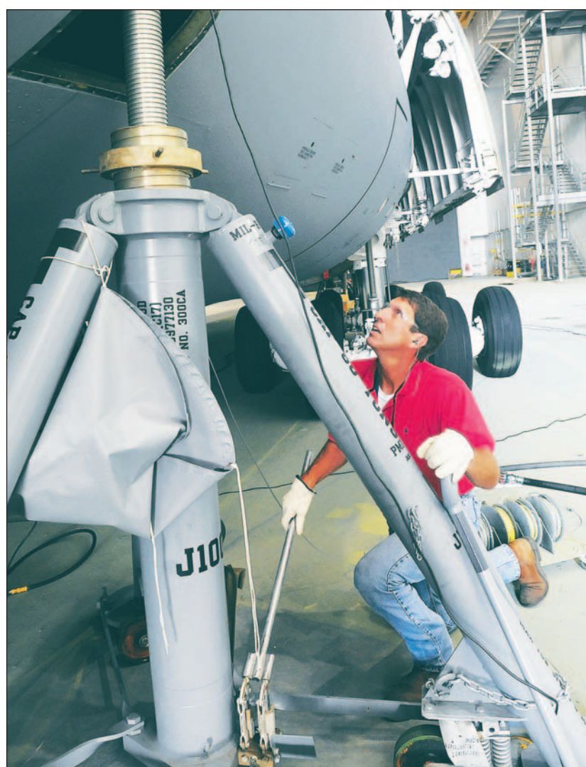
U.S. Air Force photo by SUE SAPP Hubert Watford, C-5 mechanic, uses a hand jack to level the jackstand before a C-5 is lifted for weighing.
