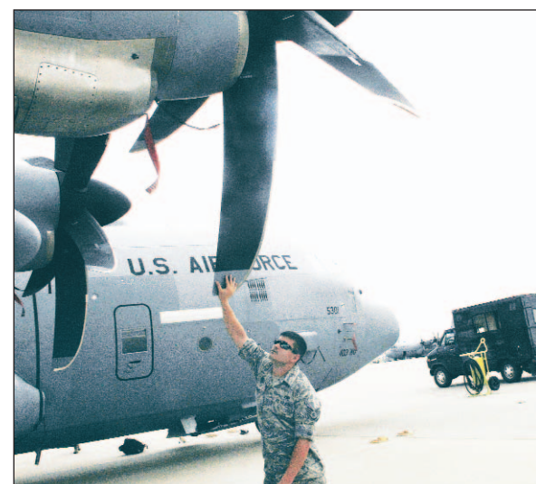
U.S. Air Force photo by SUE SAPP Staff Sgt. Damian Hebert inspects the nickel guard on the leading edge of a C-130J propeller blade.
