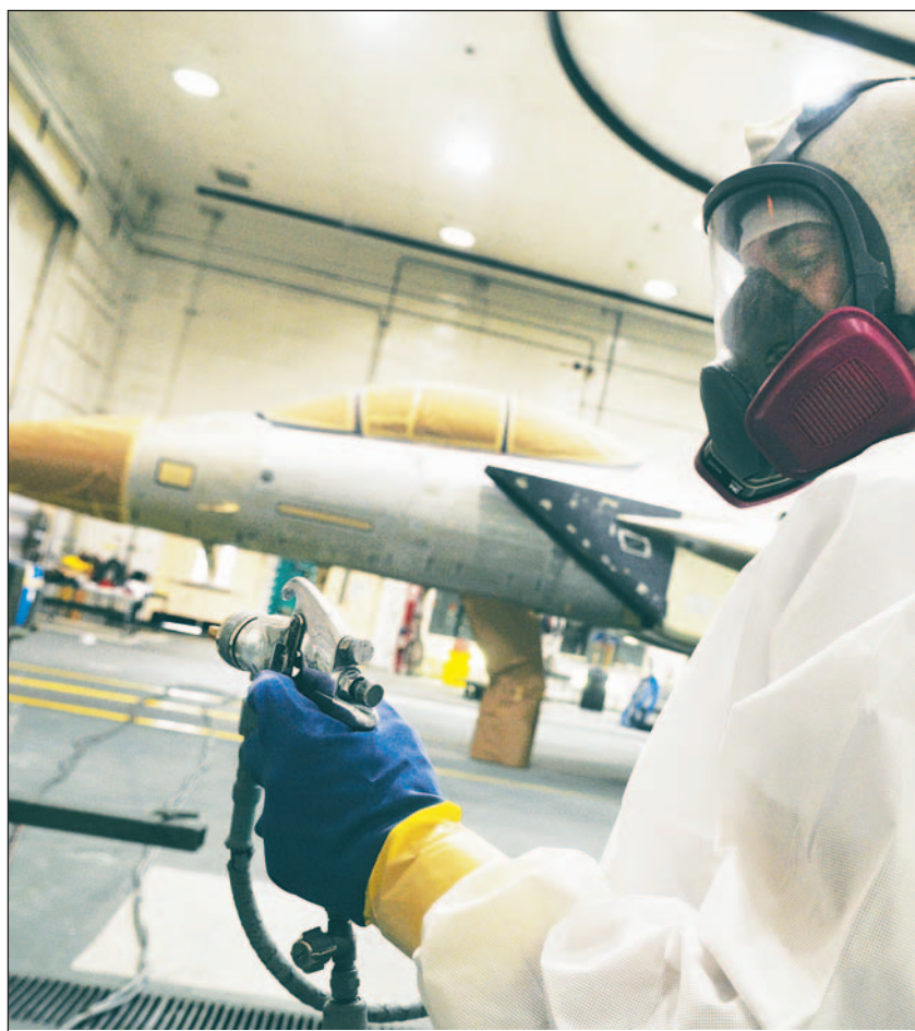
U.S. Air Force photo by SUE SAPP Chris Spivey, aircraft painter, prepares a spray nozzle before applying primer to an F-15.
