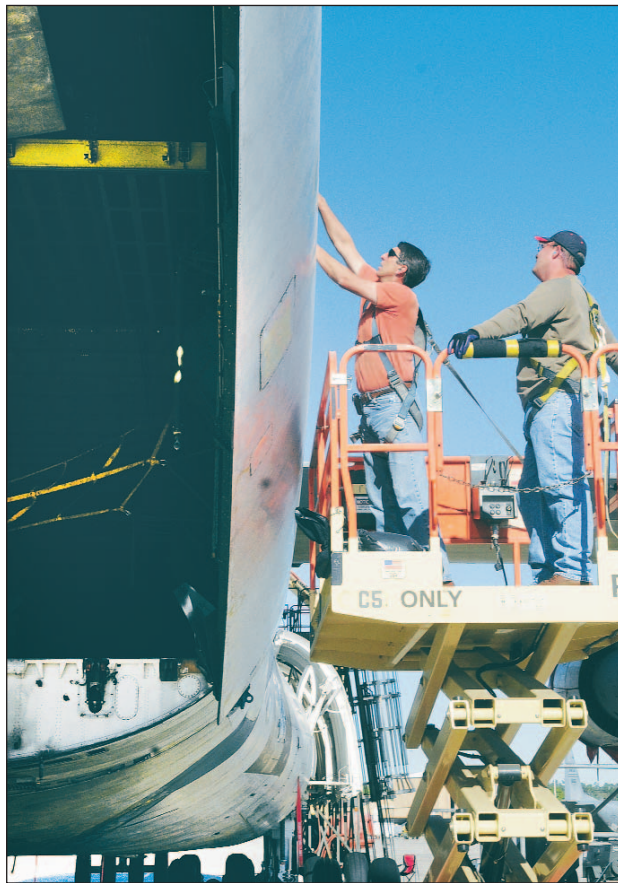
U.S. Air Force photo by SUE SAPP C-5 maintainers Hubert Watford and Sean Bohannon install an aft right cargo door.
