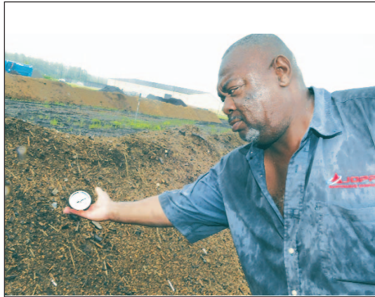
U.S. Air Force file photo by SUE SAPP Milton Fuller, compost site operator, checks the temperature of a heap of compost to see if it needs to be turned.
