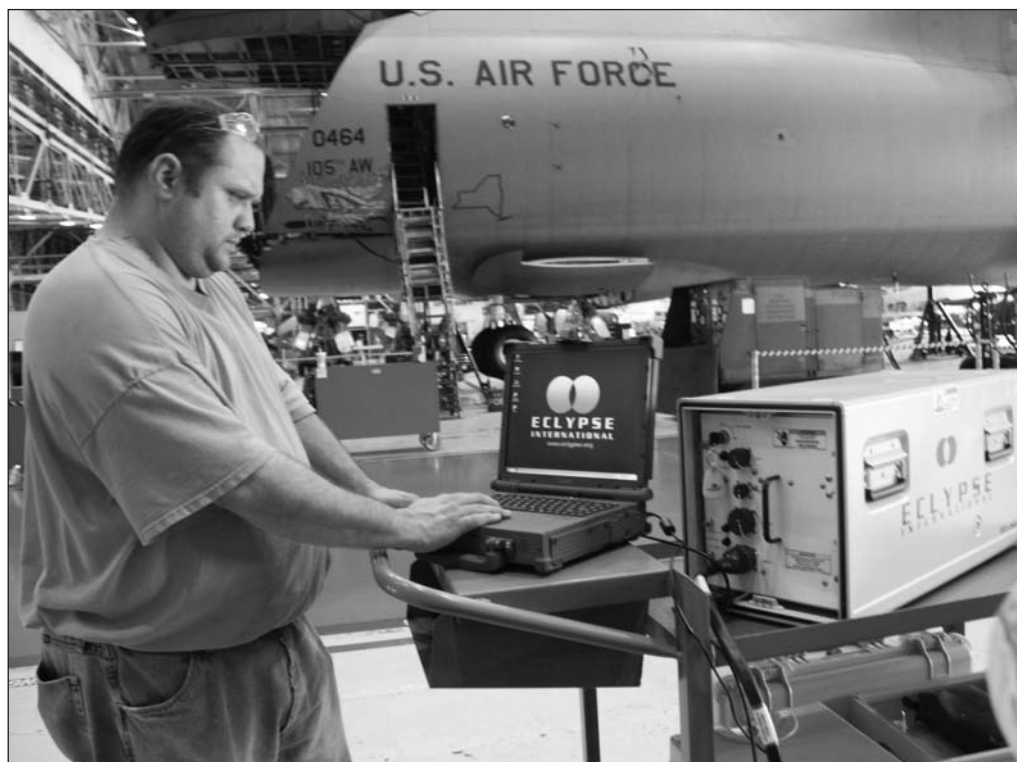
Matt Simpson, aircraft electrician, works with the new automatic wire test set.
