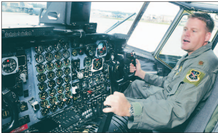
U.S. Air Force file photo by SUE SAPP Maj. Jeremy Mickelson, C-130 pilot, talks from inside the cockpit of a C-130. The C-130 Avionics Modernization Program will replace the cockpit's current display with digital gauges.
