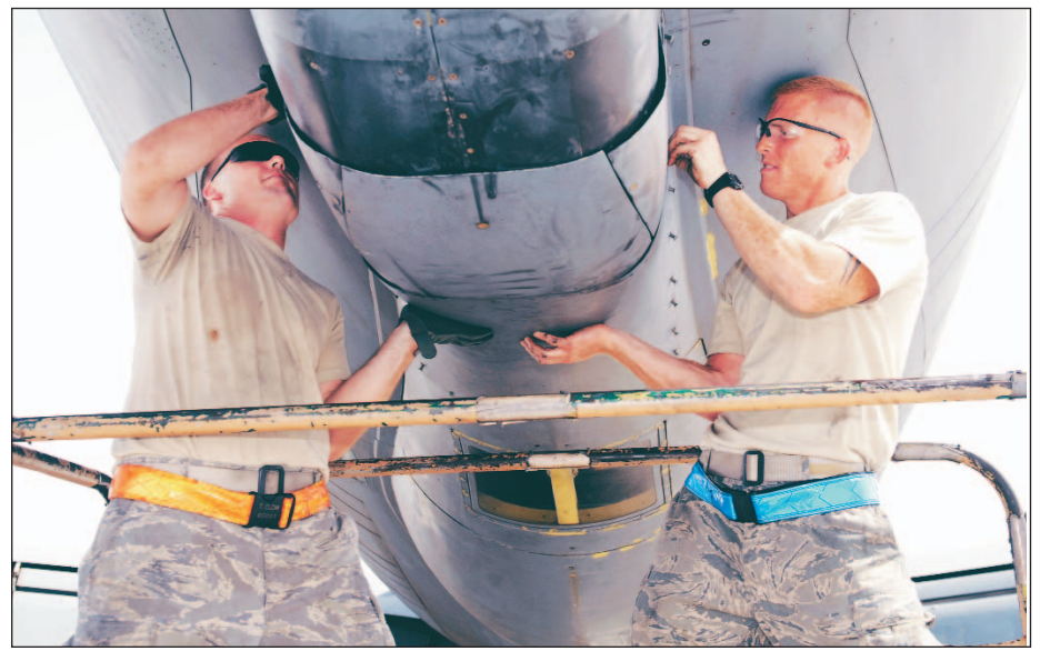
U.S. Air Force photo by TECH. SGT. MICHELLE LARCHE Tech. Sgt. Todd Clow and Senior Airman Christopher Hughes, hydraulics technicians with the 379th Expeditionary Aircraft Maintenance Squadron, attach a boom pod panel to a KC-135 Stratotanker at an air base in Southwest Asia.
