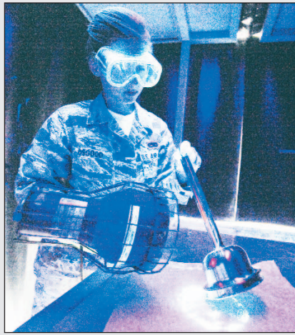
U.S. Air Force photo by SENIOR AIRMAN DANA HILL Airman 1st Class Danna Osgood, with the 1st Equipment Maintenance Squadron Non-Destructive Inspection shop, checks an F-15 Eagle hydraulic component for cracks at Joint Base Langley - Eustis, Va.
