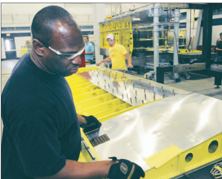
L-R, Tommie Wilder and Kevin Cranford work on a C-130 flap in the new aircraft component repair facility.
