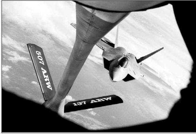
U.S. Air Force photo by STAFF SGT. ANDY KIN An F-22 Raptor prepares to receive fuel from a KC-135 Stratotanker near Andersen Air Force Base, Guam.
